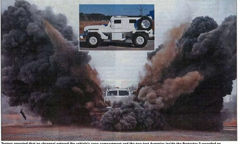
Testers reported that no shrapnel entered the vehicle's crew compartment and the two test dummies inside the Protector 2 recorded no potentially serious injuries after 6.8kg of TNT was detonated under the vehicle's hull. INSET: The Protector 2.
